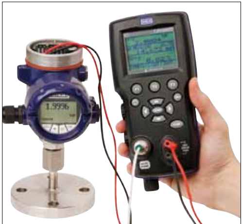
Fig. 26: Calibration of a pro- cess transmitter with portable calibrator
