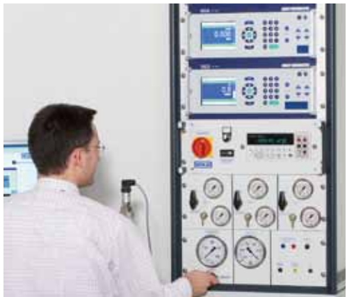
Fig. 17: Automated calibration of pressure measuring instruments
