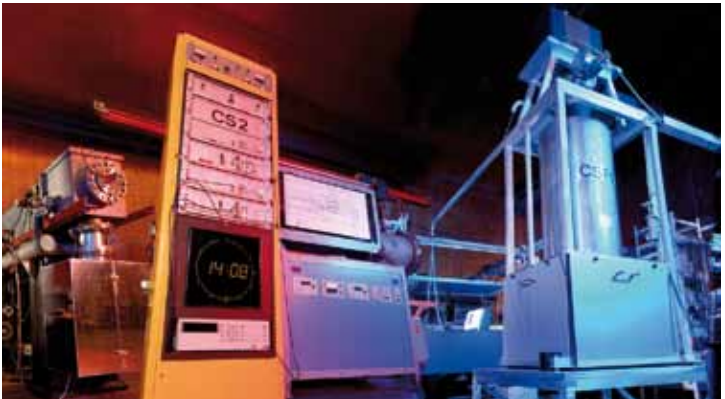
Fig. 4: Atomic clock of the PTB (German national metrology institute)
