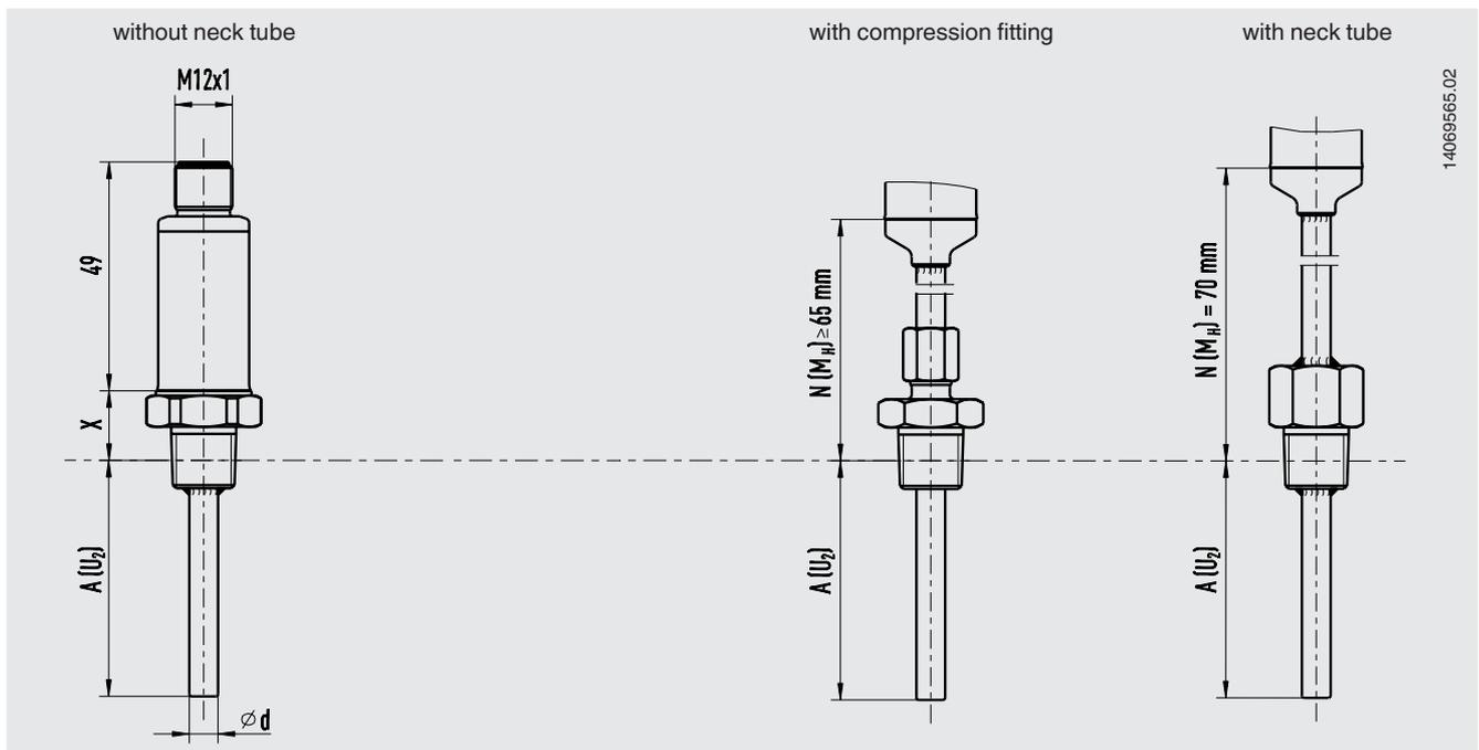
1) At a process temperature of > 150 °C [302 °F], a neck length N (MH) of 70 mm is necessary, otherwise N (M<sub>H</sub>) selectable (55, 65 or 70 mm).
